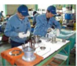
Even for an excellent pump, degradation and wear of the parts are unavoidable depending on the operating condition and operating hours. The best operation condition can be maintained for a long time by a repair and exchange of the parts at periodical inspection. Adequate support, backed by our experience and data, is quickly available in case of accident. We determine the cause of trouble and propose preventive measures.
